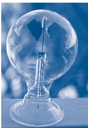
Photo 29.1 Crookes' radiometer with the black and white vanes clearly visible.
