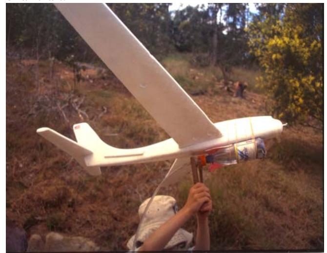
For this type of aircraft you will find that the thrust force has to be reduced by reducing  $A$ . Otherwise, the wings get ripped off the plane at take-off.
