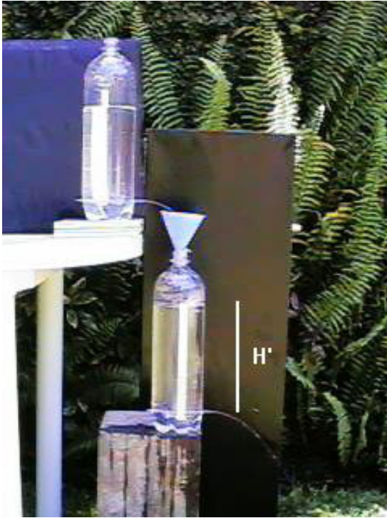
Figure 2. Two-bottle experiment, where the water flowing from the first bottle is caught by the second through a funnel. Successive heights H' were measured as a function of the time.
