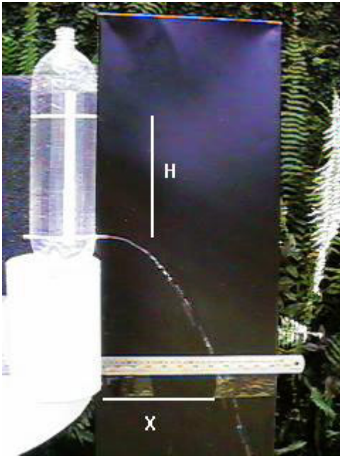
Figure 1. Experimental apparatus used in our test of Torricelli's law. Successive values of the height H were read off from a scale previously glued on to the bottle surface, with points 0.5 cm apart from each other. The corresponding speed of the water flowing at the pin-hole was indirectly measured using the distance X read off the horizontal rule. Successive times T were also measured during the flow.
