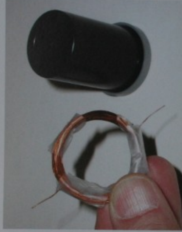
50 turns of wire and the 35 mm film canister used as a coil former.
