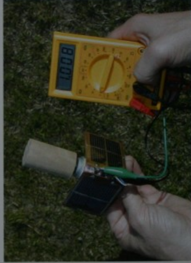
Spinning shaft voltage measurements of "Inverted Sun Compass".
