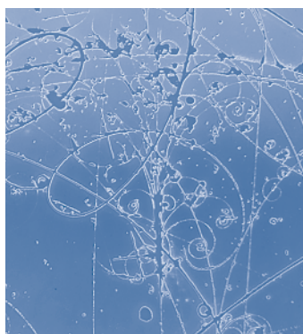
Figure 28.5 Path of an ionising particle in a spark chamber.
