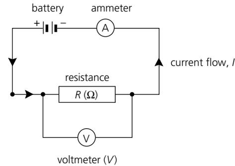
This circuit measurement depends on the relationship between applied voltage and subsequent electric current through the resistance, which is known as **Ohm's law** and which is discussed more fully in Section 22.5, but is stated as:
