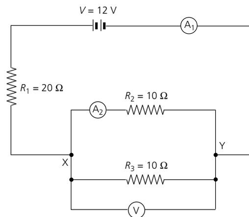
Consider the circuit drawn in Figure 22.16 containing a simple network of three resistors connected to a DC battery of 12 V. Use circuit laws to calculate the readings on the electric meters in the circuit.
