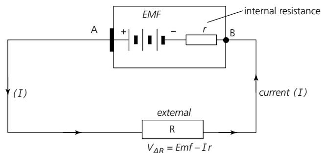
Figure 22.11 shows the circuit diagram for a battery supplying current to an external resistance,  $R$ , and includes the battery's internal resistance. Because the current,  $I$ , passes through the battery as well, a potential drop of  $Ir$  is caused, which subtracts from the battery EMF. Thus the terminal voltage of the battery, as measured by a voltmeter, would be:
