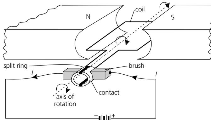
but contains a special switch assembly on the rotating coil shaft that allows the direction of the current through the coil to be reversed every  $180^\circ$ . This switch is called a **split-ring commutator** and is shown in simplified form in Figure 25.28.
