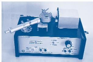
Millikan studied the behaviour of thousands of oil drops and was able to work out the charges on them. He found that all charges were whole-number multiples of the minimum charge of  $1.602\ 1892 \times 10^{-19}$  coulombs. It is worth remembering that an uncharged oil drop still has billions of electrons but these are balanced by an equal number of protons. In Millikan's experiment, it is the *excess* electrons that are being counted.
