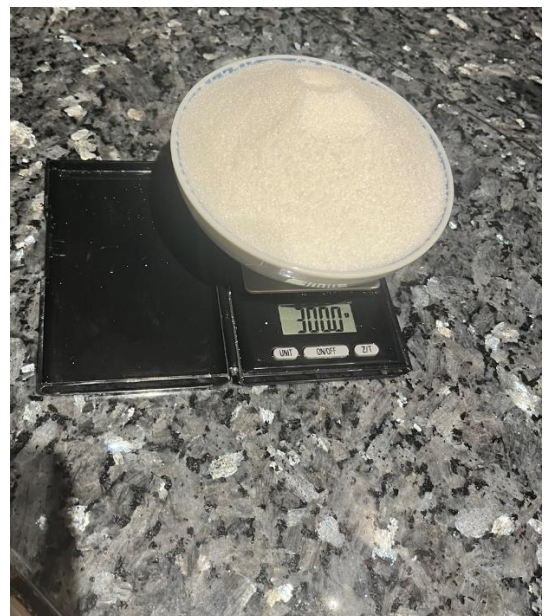
Figure 5: Measuring 300g of sugar to make 30% sucrose solution
