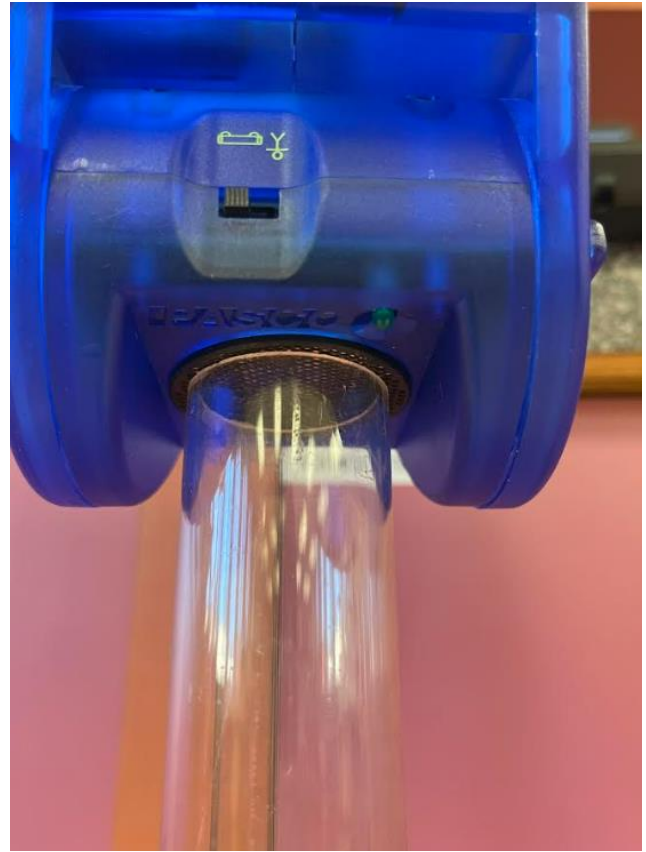
Figure 3: a closer look at the motion sensor on top of the tube
