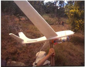
For this type of aircraft you will find that the trust force has to be reduced be reducing *A*. Otherwise, the wings get ripped off the plane at take-off.
