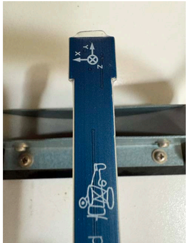
You can choose the field direction for the sensor. I used the y-direction at right angles to the plane of the loop (parallel to the field).
