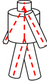
Figure 1: Six element NEC wire model of the human body.
