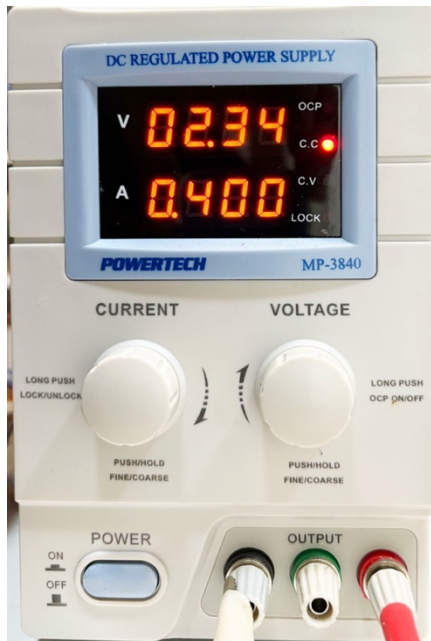
Regulated power supply set to a current of 0.400 A
